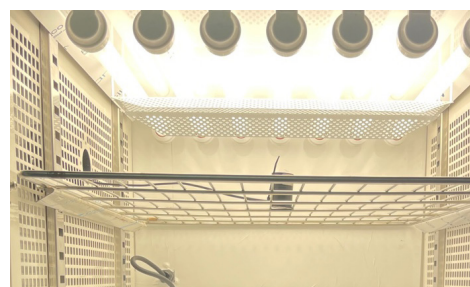
Specially manufactured filter for uniform illuminance
